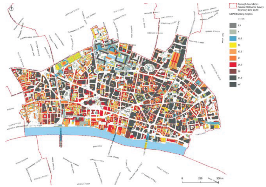
For an illustrative comparison, building heights in 2020 using LIDAR data coloured to approximate storey heights. Note also the change in plot sizes.
