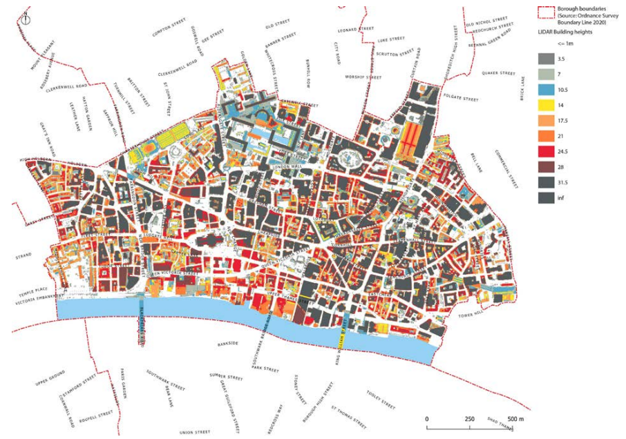
For an illustrative comparison, building heights in 2020 using LIDAR data coloured to approximate storey heights. Note also the change in plot sizes (© Alan Baxter)
