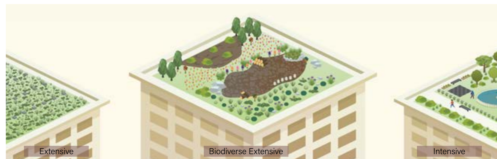
Figure 7.1: Types of greenroofs
