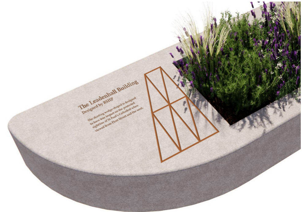
Brass inlays to planter top (illustrating the triangulated forms of the Leadenhall Building's megastructure)
